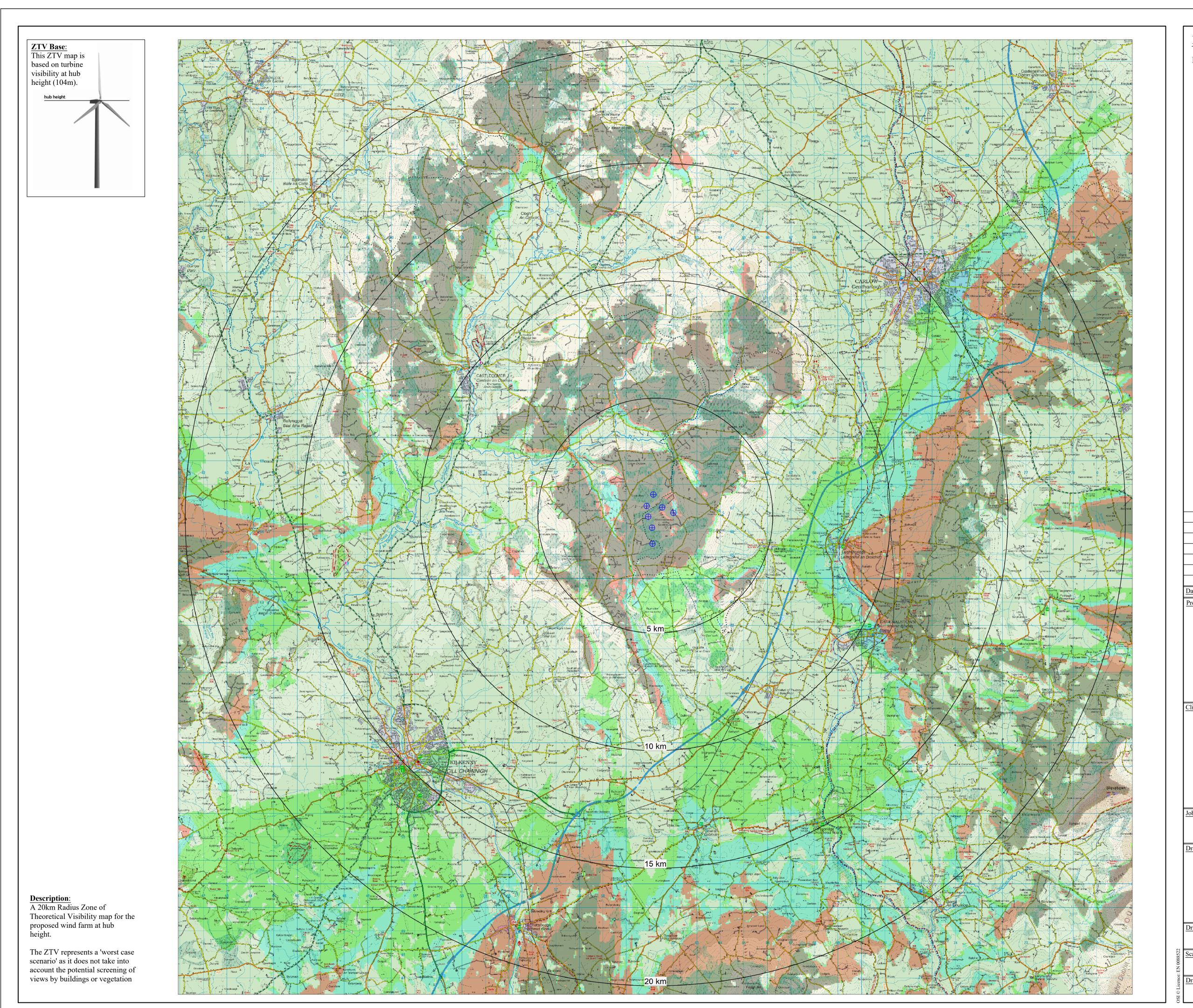
**Legend:** Proposed Wind Turbines Locations Number of turbines theoretically visible 1 to 2 3 to 4 5 to 6 Drawn By: Date:Rev:Description: Prepared by: GALETECH ENERGY SERVICES Galetech Energy Services, Clondargan, Stradone, Co. Cavan White Hill Wind Limited White Hill Wind Farm Drawing Title: Figure 144: ZTV map at hub height Drawing No.: Revision No.: WHI001\_PAS\_PHO\_04 (A1) 1:75,000 25/10/2022 Checked By: Confirmed By: C.M.P. S.C
